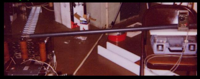
Here is the unwieldy finished product, covered with PVC heat-shrink tubing, balanced on my <u>Cockcroft-Walton voltage</u> <u>multiplier</u>.
