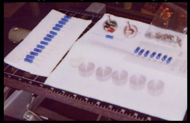
This picture shows the parts ready for assembly. The polycarbonate disks were cut with a router and compass attachment. The fiberglass tubing was cut with a carbide hacksaw blade and the end trued and trimmed with a Dremel rotary tool with diamond cut-off wheel (glass dust everywhere, seriously itchy too). The six holes through the fiberglass tube for the end cap mounting screws were drilled with a 3/16" titanium nitride coated drill bit and counter sunk with an 82° high speed steel bit.
