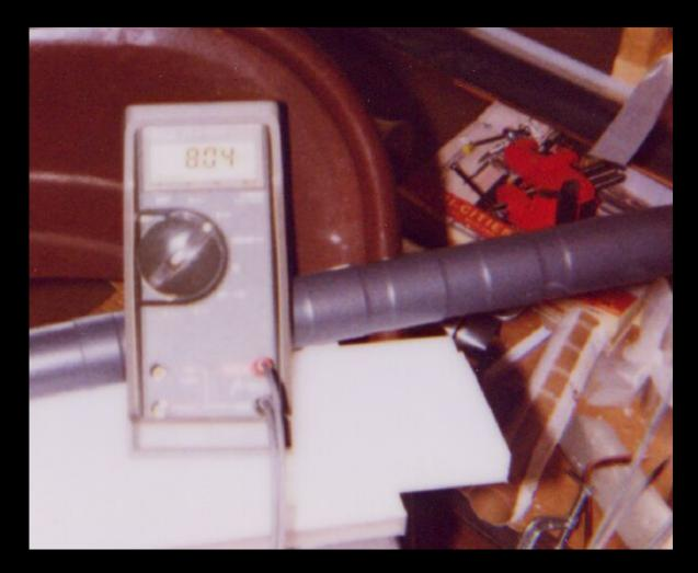
In this photo, you can see the ribbed handle of the probe and the read-out of 80,400 (8.04 X 10,000) volts from the C-W.
