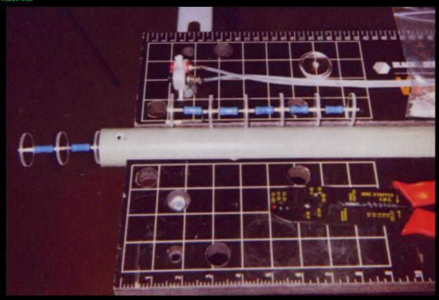
This photo shows the parts being put together. Most of the resistors are in the tube (except for the five assembled above the tube and four which were still on back-order from Newark when this picture was taken). Also shown are the two 24" insulated leads which will run through the handle and are soldered to the banana jacks (which are color coded so I can't screw up and put 500,000 volts through my multimeter) [10/20/01: the banana jacks were replaced with a BNC bulkhead jack].
